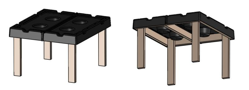
**5)** The base can now be secured to the frame by driving screws or nails through the sides of the base and into the wood frame. There is no need to predrill holes.
